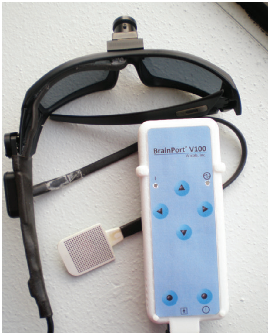
Figure 1. BrainPort consists of a pair of sunglasses (with an integrated video camera), a 20 × 20 array of stainless steel electrodes that is placed on the tongue, and a handheld computer that processes the video camera's input, contains contrast and stimulation intensity controls, and activates the electrode array.
